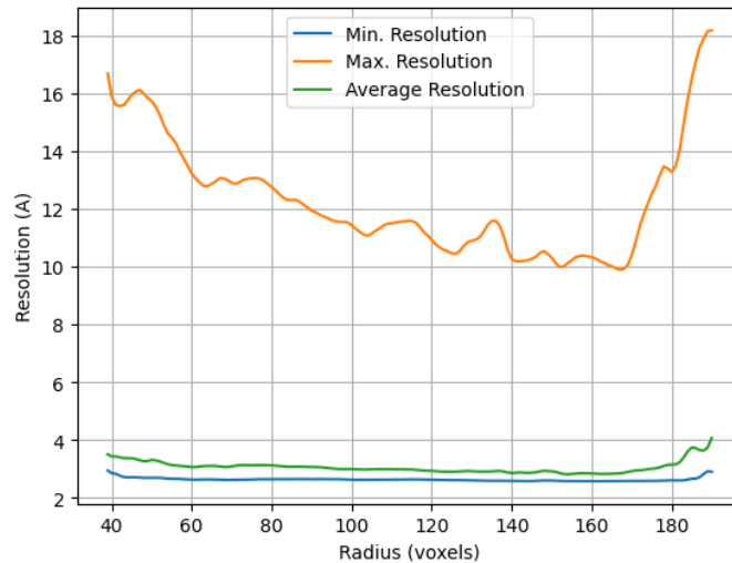
Figure 27: Radial averages (in space) of the minimum, maximum and average resolution at each voxel.
