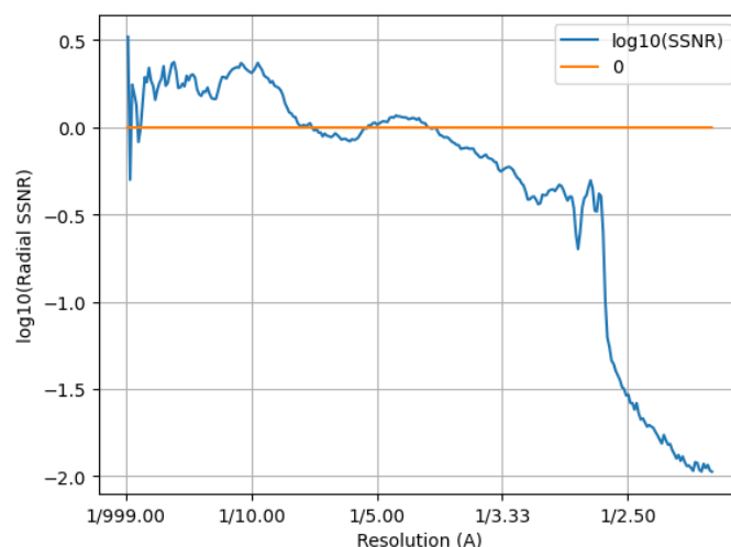
Figure 21: Spectral Signal-to-Noise Ratio estimated from the two halves.
